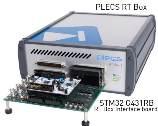
Figure 8: Hardware setup for the HIL verification
