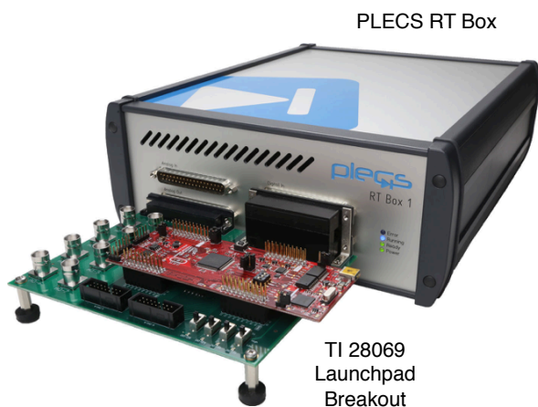
Figure 7: Hardware setup of the HIL verification
