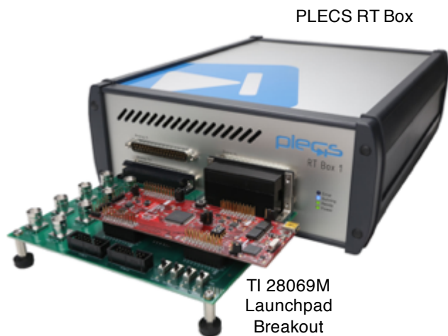
Figure 4: Hardware setup of the HIL verification with the RT Box
