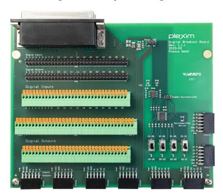
Figure 2.1: RT Box Digital Breakout Board
