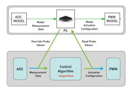
In PIL mode, values calculated by the simulation tool are used as inputs to the embedded algorithm, instead of reading the physical sensors. Similarly, outputs of the control algorithms executing on the processor are fed back into the simulation to drive the virtual environment.
