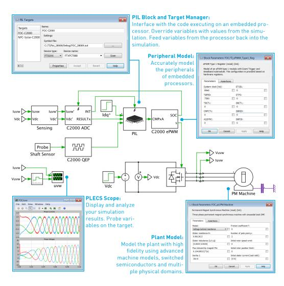
PLECS® is the tool of choice for high-speed simulations of power electronic systems. It is available in two editions: PLECS Blockset for seamless integration with MATLAB®/Simulink®, and PLECS Standalone, a completely independent product. PLECS PIL is licensed as a separate feature.
