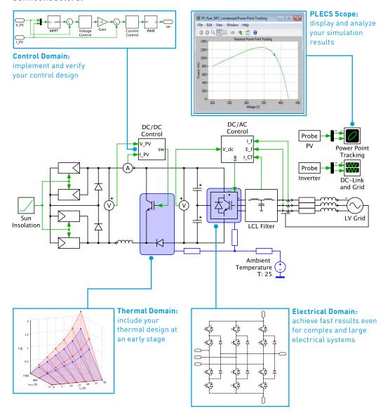
PLECS® is the tool of choice for high-speed simulations of power electronic systems. It is available in two editions: PLECS Blockset for seamless integration with MATLAB®/Simulink®, and PLECS Standalone, a completely independent product.
