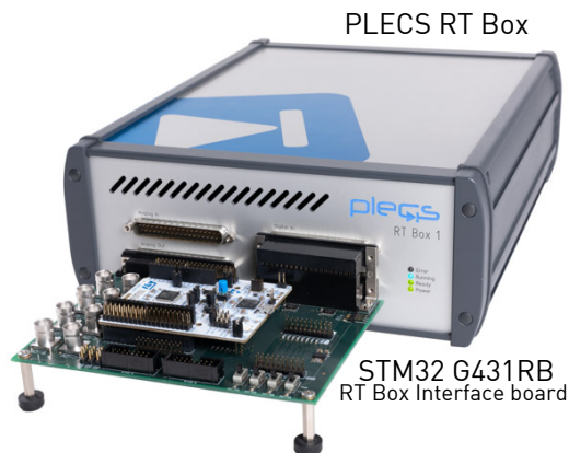
Figure 8: Hardware setup for the HIL verification
