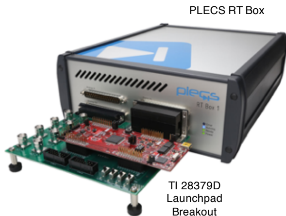
Figure 8: Hardware setup of the HIL verification
