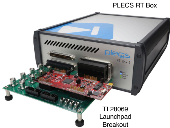
Figure 6: Hardware setup of the HIL verification with the RT Box
