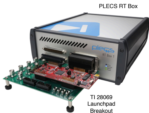
Figure 7: Hardware setup of the HIL verification
