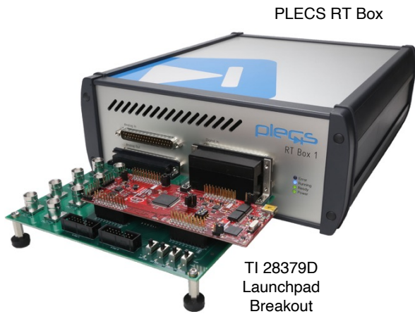
Figure 12: Hardware setup of the HIL verification
