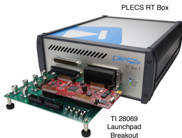
Figure 7: Hardware setup of the HIL verification
