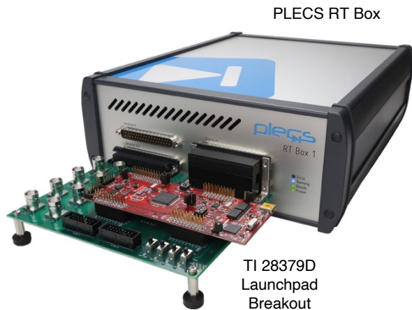
Figure 12: Hardware setup of the HIL verification
