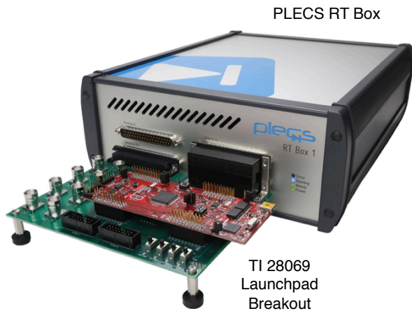
Figure 6: Hardware setup of the HIL verification
