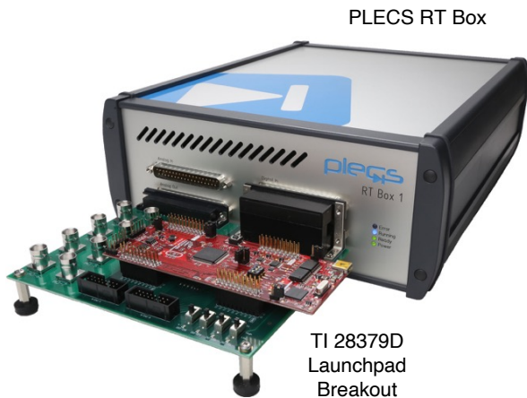
Figure 12: Hardware setup of the HIL verification
