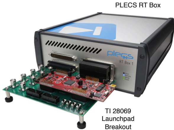
Figure 6: Hardware setup of the HIL verification
