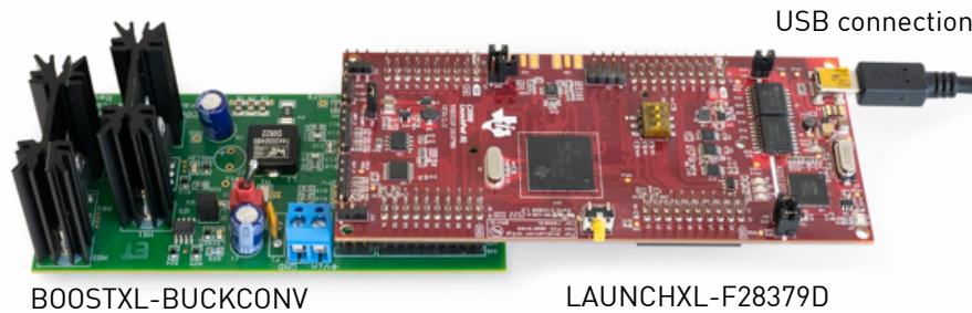
Figure 7: Hardware setup of the BOOSTXL and TI C2000 Launchpad
