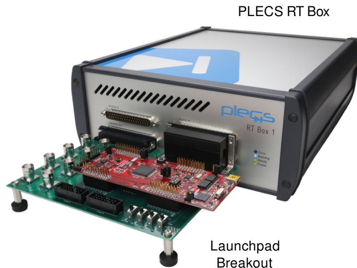
Figure 9: Hardware setup of the HIL verification with the RT Box
