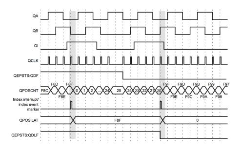
The figure below shows the operation of a 1000-line encoder with QPOSMAX set to 3999 and operated in PCROI mode.
