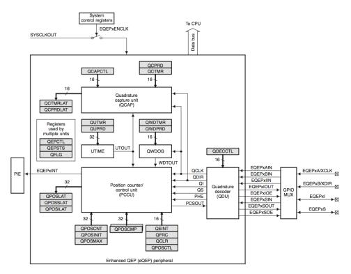
Functional Block Diagram of the eQEP Peripheral [1]
