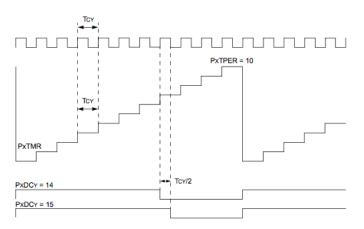
Duty cycle resolution timing diagram, Free Running mode, and 1:1 prescaler selection [1]
