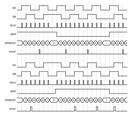
Position counter underflow/overflow (QPOSMAX = 4) [1]
