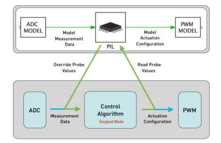
At the most basic level, a PIL simulation can be summarized as follows:
