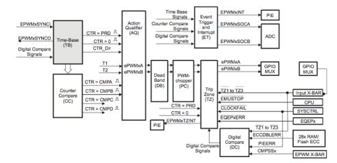
The ePWM type 4 module consists of several submodules:
